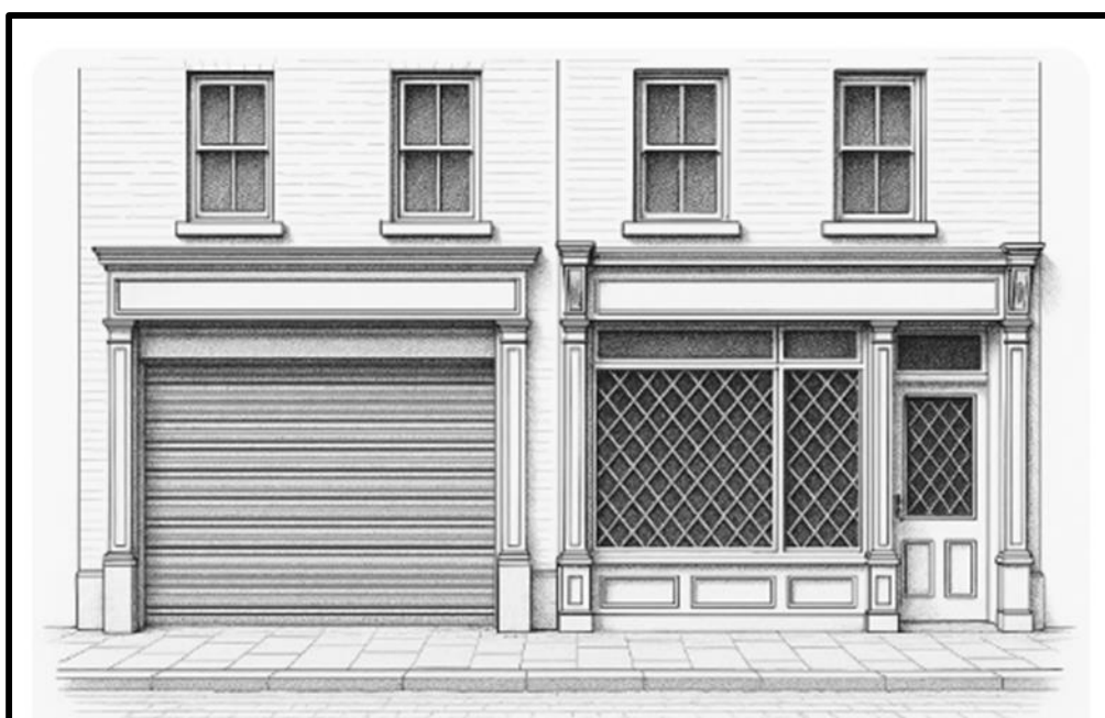
Figure 3: Examples of unacceptable shutters (left) and adjacent acceptable internal security grille (right)
